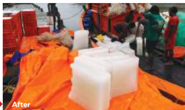
Ice blocks kept on polysheets avoiding surface contact
